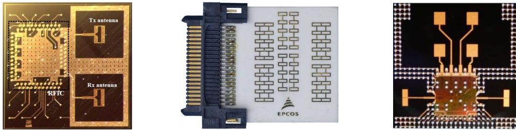
(a) 硅基射频微系统 (a) Silicon-based RF microsystem (b) 陶瓷基射频微系统 (b) Ceramic-based RF microsystem (c) 树脂基射频微系统 (c) Resin-based RF microsystem
