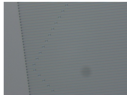
图 1 光刻后的 Pt 样品表面 Fig. 1 The Pt sample covered with patterned photoresist
